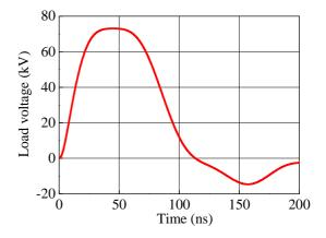
**Figure 8.** Simulated load voltage at RL = 1 Ohm at 200 kV charge voltage on the capacitors.
