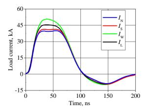
**Figure 12.** Load current measured by separate B-dot probes, and the total load current  $I_L$  calculated by using Eq. 14. Same shot as that in Fig. 11.
