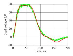
**Figure 13.** Recorded (in green) and simulated (in red) load voltage at *s*=4, *m*=2,  $R_L$ =1.65 Ohm, at  $U_{CH}$  =±100 kV. The current loop around the core is broken, the resistance of the core is set to RC =10<sup>6</sup> Ohm.
