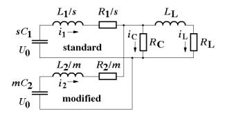
**Figure 3.** Simplified electrical scheme of the Square Pulse LTD.
