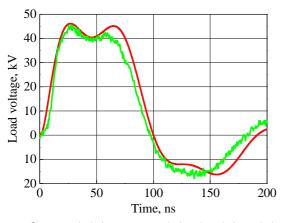
**Figure 9.** Recorded (in green) and simulated (in red) load voltage at s=m=2,  $R_L=1.65$  Ohms, at  $U_{CH}=\pm96$  kV.
