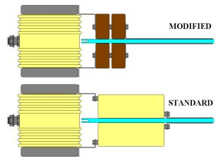
**Figure 5.** Modified brick with TDK ceramic capacitors and standard brick with GA 35460 oil-filled capacitors.
