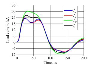
**Figure 10.** Load current measured by separate B-dot probes, and the total load current  $I_L$  calculated by using Eq. 14. Same shot as that in Fig. 9.
