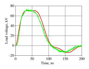
**Figure 11.** Recorded (in green) and simulated (in red) load voltage at *s*=4, *m*=2,  $R_L$ =1.55 Ohm, at  $U_{CH}$  =±100 kV.
