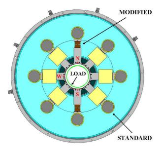
**Figure 4.** Square Pulse LTD with 6 standard and 2 modified bricks.
